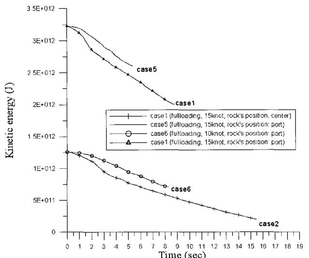
Fig. 22 Comparison of kinetic energy reduction (case 1,2,5,6)
