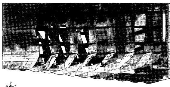
Fig. 19 Damaged shape of web frame for case 5,6
