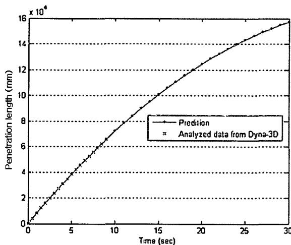
Fig. 23 Prediction of penetration length by quadratic-polynomial method
